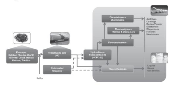
Fluorine chemistry is highly complex; however, as one of the pioneers of fluorine chemistry, we have decades of experience. To liberate elemental fluorine, we transform calcium fluorite (fluorspar ore) into hydrofluoric acid. Multiple chemical processes are then utilized to transform hydrofluoric acid into fluorochemicals, fluoroplastics, fluoroplymers, fluoromonomers, fluorotelomers, fluoroelastomers, films, membranes and coatings.
